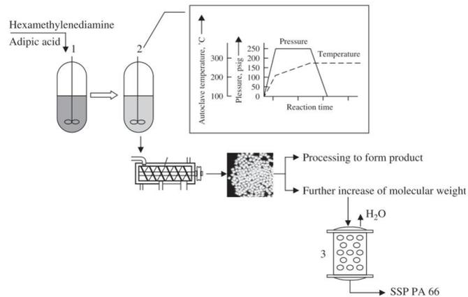
**Figure 1:** Industrial production of PA66 with SSP finishing step.
